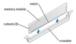
**NOTICE:** To avoid damage to the memory module, press the module straight down into the connector while you apply equal force to each end of the module.
